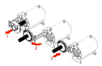
Figure 34: Burner Door Opening
