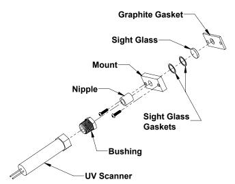
Figure 33: UV Scanner Assembly
