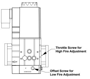
Figure 30: Gas Valve Air/Fuel Adjustment
