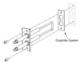
Figure 31: Igniter Electrode Assembly
