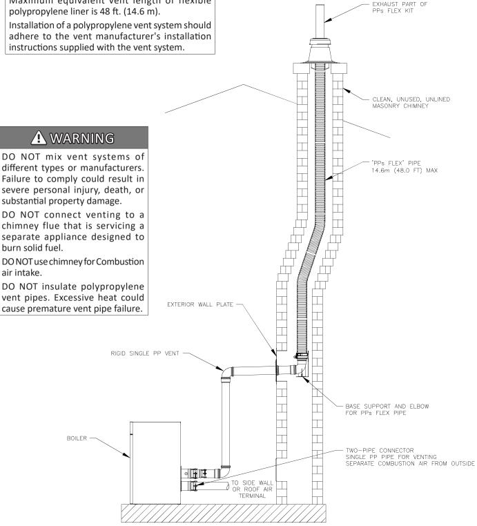
Figure 10: Flexible Vent in Masonry Chimney with Separate Combustion Air Intake
