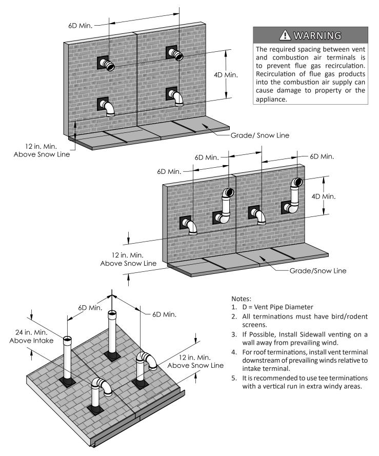
Figure 9: Multiple Appliance Direct Vent Termination
